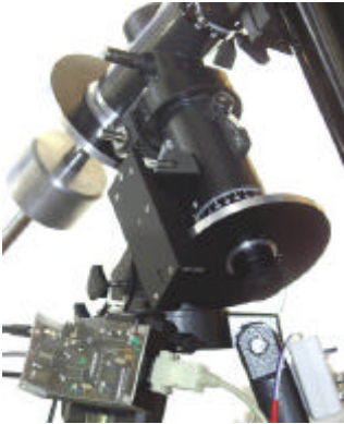
Figure. 7. a, b. Sensor, parts their placing and fixation on mount GS 300. On Al disc surface of 100 mm radius fixed on axes DE, white matt office impregnated paper is stuck , A Screw with denticulated head on back wall of sensor IRC-M adjusts position of the sensor to the disc, i. e.. radius size -of scan circle and its corresponding number pulse. Number of pulses/360° must be identical with arithmetic pulse defined in SW single-chip MCU-CITAC in modulus NAVIGATOR-1.
