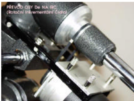
Figure 3. (jpg) close-up view of axes De on IRC strap transmission and IRC fixation to mount with the help of two lengthwise steel mouldings Al profile with IRC fixed directly on them.
